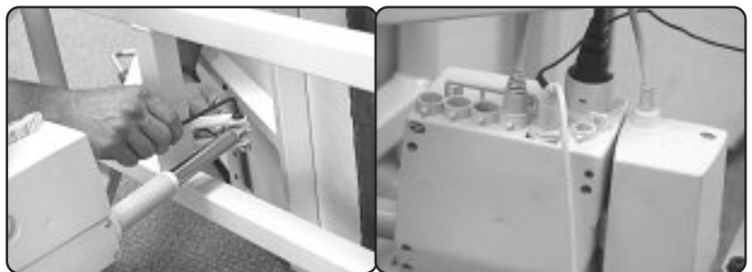
Re-attaching the Motor Actuator
